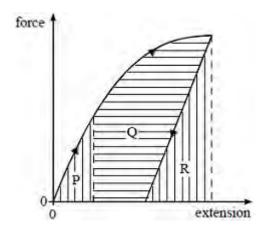
The increase in thermal energy in the sample is represented by area
