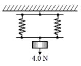
The spring constant of each spring is 20 N m<sup>-1</sup>. The elastic energy, in J, stored in the system is
