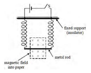
When both the spring constant and electrical resistance of **each** spring is doubled, closing the switch would now cause the rod to be displaced a distance
