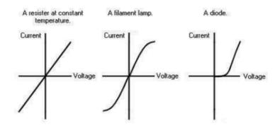
In a filament lamp, this is because as the **current increases** through the filament, so does the **temperature**, which means **electrons and ions vibrate more** and **collide more**, **increasing resistance**.
