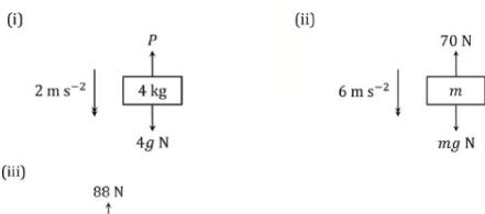
For motion in a straight line, F = ma (Newton's Second Law of Motion)
