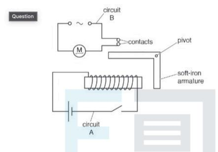
Circuit A contains a switch that operates the motor in circuit B when it is closed.
