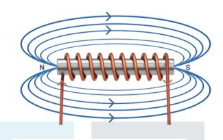
2. If you uncoil a solenoid, it becomes a straight wire. When current flows through this wire, it generates a magnetic field around it.
