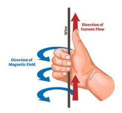
The right-hand grip rule helps determine the direction of the magnetic field around a current-carrying conductor, where the thumb points in the direction of the current and the curled fingers indicate the direction of the magnetic field lines.
