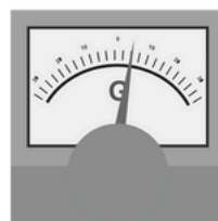
GALVANOMETER • USE TO MEASURE TINY CURRENT
